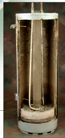
Example of mineral buildup in an unprotected water heater.
